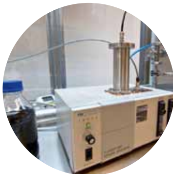
Figure 2.3 Generator to aerosolize carbon nanotubes. (Photo by Joonas Koivisto, FIOH).
